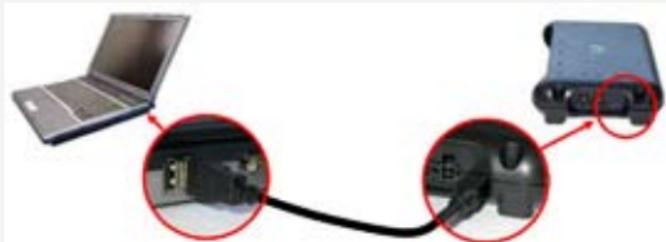
1. Connect the central unit to the computer using a USB cable (USB A to USB mini B)
