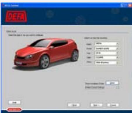
4. Choose car Make, Model, year, type and other. When all the choices have been made the "Show"-button is accessible. Pressing this button will show the installation guide for the chosen car, which can be printed if necessary
